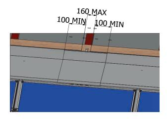
In the same way, place the corner flashings, having applied beforehand a PU glue joint on the overlapping zone of the top flashing. (Overlapping at least 100mm)
